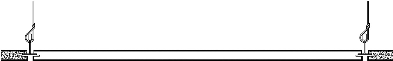
STEP 3: SLIDE PANEL TO RIGHT TO LOCK PANEL ONTO GRID
