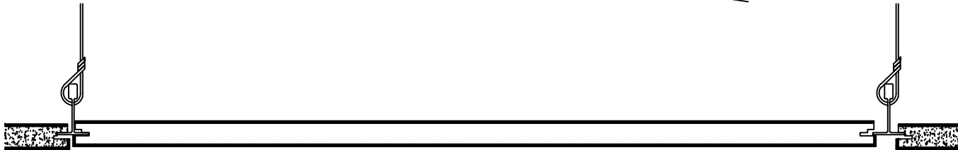
STEP 2: SLIDE PANEL TO LEFT TO ALLOW SOUTH EDGE TO CLEAR
